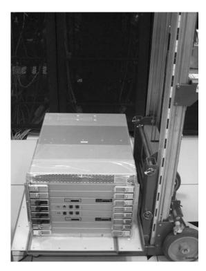
Figure 11. Lift tool and chassis positioned at rear of cabinet
